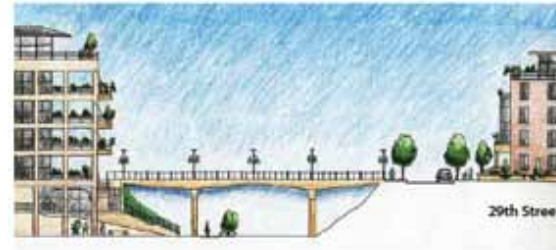
Section AA: Midtown Greenway: Buildings on the north side of the Greenway should either engage the Greenway at the lower level with workspaces and residences or should be set back on the upper level to create a public edge and overlooks.
